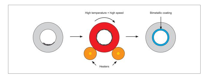
Both bimetallic and bimetallic plus products are the same nitrited and got the same chrome plating layer. The difference is in production manufacturing and composition of bimetallic powder alloy.
